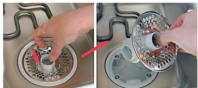
Figure 5-4: Pump filter removal
